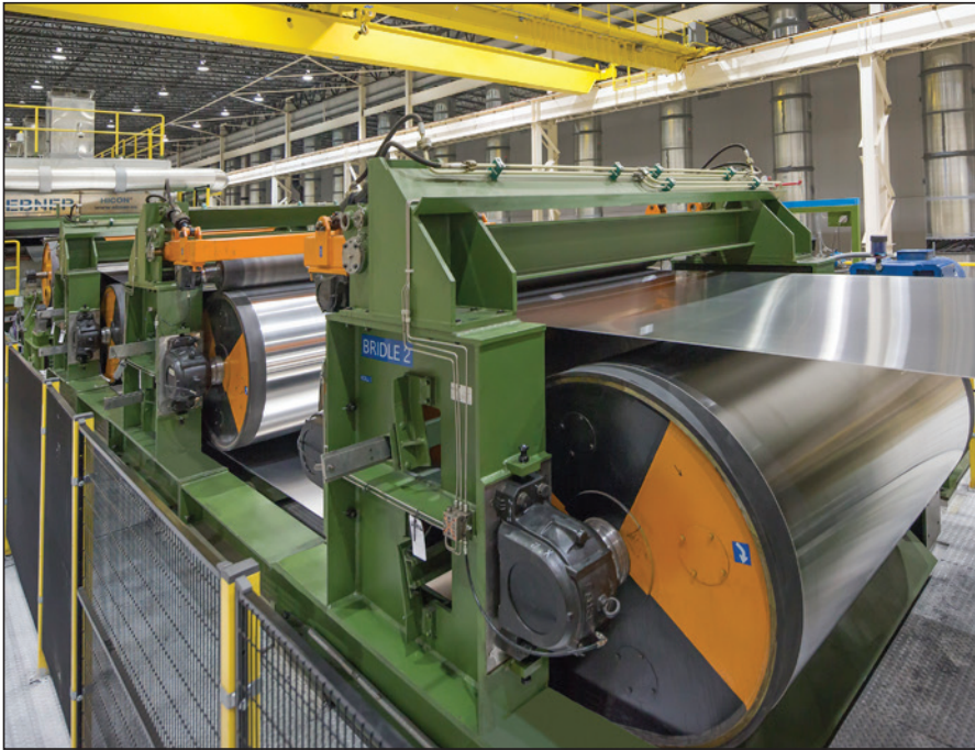
Close-up view of the aluminum sheet exiting Bridle 2 on the new CASH line at the Oswego facility.
