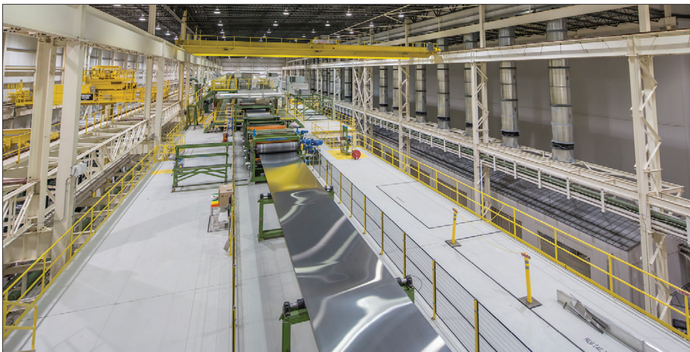
Overall view of the CASH 3 finishing line for automotive aluminum sheet in the new building at Novelis' facility in Oswego.
